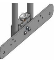
Now the rail is ready to be installed onto bed. Insert long countersunk screws through mounting plate and bed spacers
