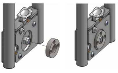
2. Use an Allen key to install the three washers and screws through the circular spacer. Do not overtighten screws
