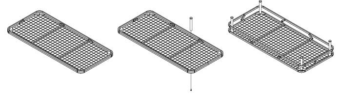
Gently pull the frame apart and install desired corner pieces on all four corners using the push in clips. Use tall corner pieces for tall upholstery option or short corner pieces for short upholstery option.
