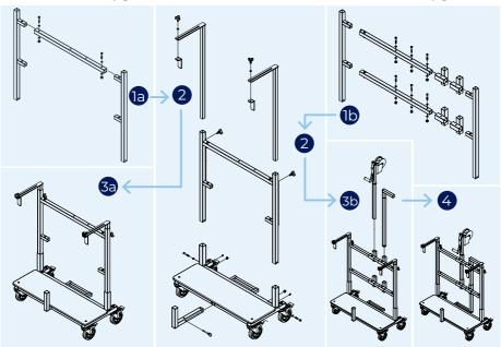
Assemble the uprights to the cross bar and lock in place using bolts, washer and locknuts. **b** If installing the winch upgrade kit: install the winch and long leg receiver tubes as shown.
