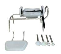
Attach the backrest by lining up the backrest frame with the holes on the main frame and inserting it. Make sure the pins slot into their holes correctly as shown in images.
